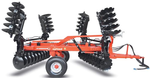
Goble type foldable trailed disc harrow is manufactured at the ranges between 18 and 56 discs and suitable to the 65-360 horsepower tractors. It cultivates the soil without clod in the dry months where plows cannot run after harvesting besides smashing the stalks of the plants like sunflower, rice and wheat and prepares the field to agriculture without requiring any other agriculture machine.
