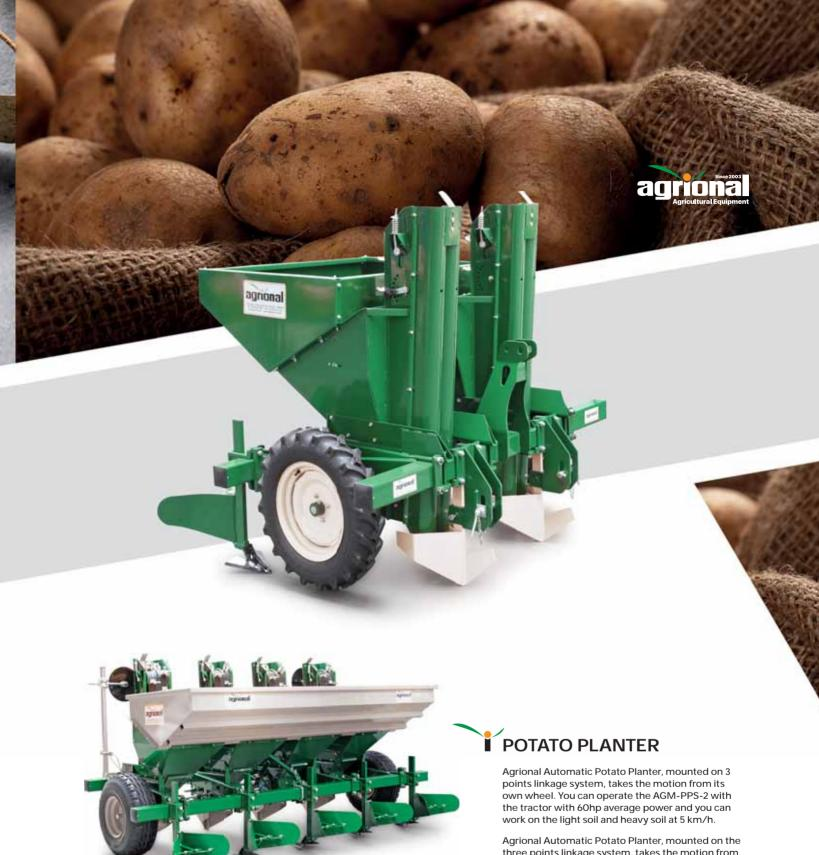
Agrional Automatic Potato Planter, mounted on the three points linkage system, takes the motion from its own Wheel. While the lump tank with 1300kg extended capacity and with bolt mounting is full, the machine's total weight is approximately 2300kg. You can operate the AGM-PPS-4 by the tractor with 60hp average power and you can work on the light soil and heavy soil at 5km/h.
